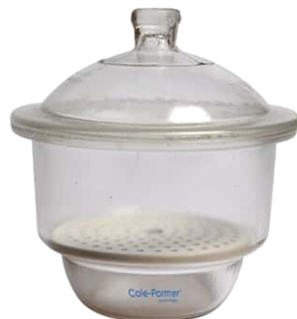
Fig 2: Bell jar with grate floor
